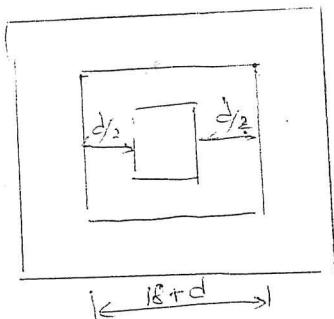
$$v_{ps} = \frac{V_u}{bd} = \frac{6.25 \times (8 \times 8 - (\frac{18+33}{144})^2)}{4 \times (\frac{18+33}{12}) \times \frac{33}{12}}$$
