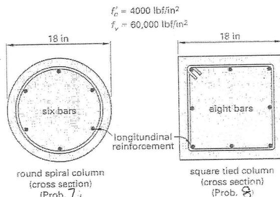
7. For the short round spiral column, the applied axial dead load is 150 kips, and the applied axial live load is 350 kips. Assuming that the longitudinal reinforcing bars are all the same size, the minimum required size of each longitudinal reinforcing bar is
