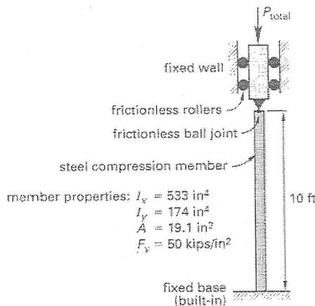
9. In accordance with American Institute of Steel Construction (AISC) load and resistance factor design (LRFD) specifications, this compression member is a
