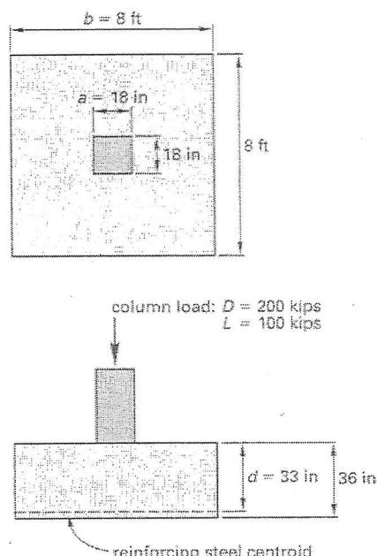
In accordance with ACI strength design, the controlling (maximum) factored shear stress is most nearly
