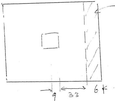
$$v_{bs} = \frac{V_u}{bd} = \frac{(6.25 \times 8 \times \frac{6}{12})}{(8 \times \frac{33}{12})} = 1.14 \text{ kip/ft}^2$$
