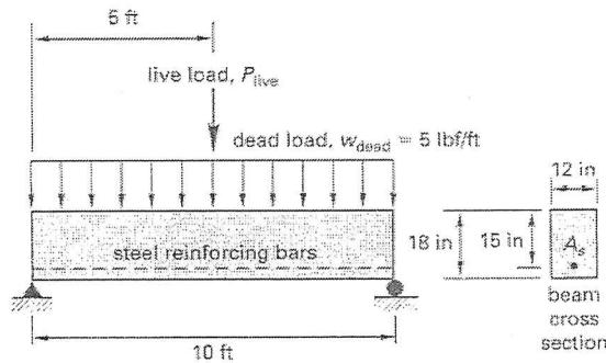
14. Neglecting beam self-weight and based only on the allowable moment capacity of the beam as determined using American Concrete Institute (ACI) strength design specifications, the maximum allowable live load is most nearly
